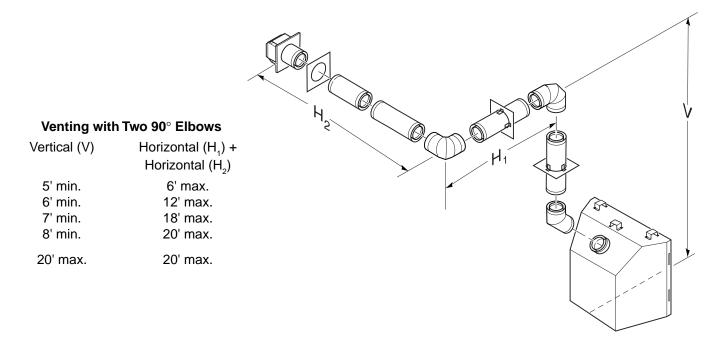
Figure 20 - Horizontal Termination Configuration for Rigid Venting Using Two 90° Elbows with Termination at 90° with Fireplace
